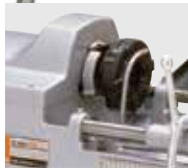
Oil lubrication system and 4 jaw vice clamping
