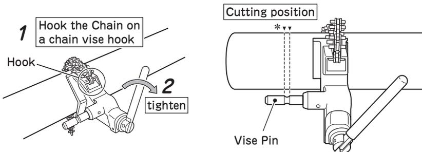
\*Cutting point varies depending on mounting position of the pipe saw.
