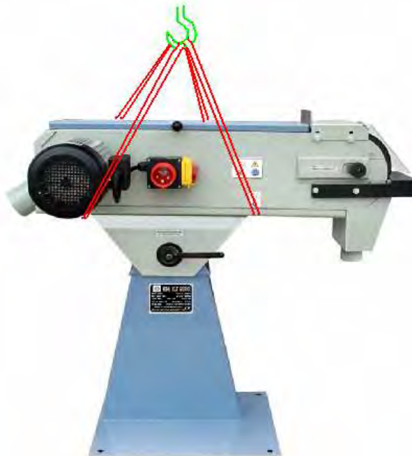
Fig. 4-2 Transportation sketch with a crane (After unpacking)
