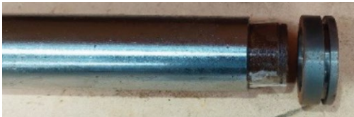
Figure 8: This pic shows the ram and collar with seals removed.
