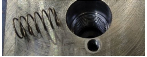
Figure 5: Control Spring removed. Note: in this picture, the right end of the spring is slightly curled in. This end must go against the small ball Figure 6.
