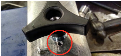
Figure 3: Control valve with retaining screw removed
