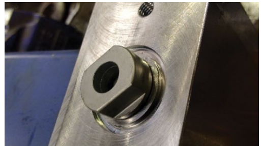
Figure 2: The primary cylinder assembly fitted.
