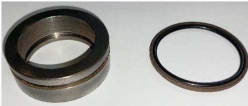
Figure 9: Collar and ram glide seal with its energising O-ring.
