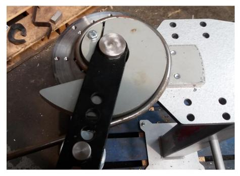
Complex Bends are achievable in Mild Steel. It will bend up to Dia ½ inch (12mm) Round and Square mild steel Bar with a minimum radius of approx 3/8 inch (10mm) Diameter and 3/8 inch (10mm) Round and Square mild steel Bar to a radius of ¼ inch (7mm)
