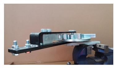
This Bender is ideally suited to be mounted along with our O64 Tube Bender on a stand such as our O65 Tube Bender Stand to make best use of the full Bending Rotation. A suitable stand setup that would allow full rotation is recommended to get the best out of this bender. If this is not possible the Tooling Disc (round Disc with all the holes on) in most cases can be easily lifted and turned 180 degrees to complete a bend.
