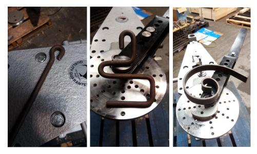
This Bender is an add on attachment to our O64 Bramley Tube Bender or can be used on its own in a vice.
