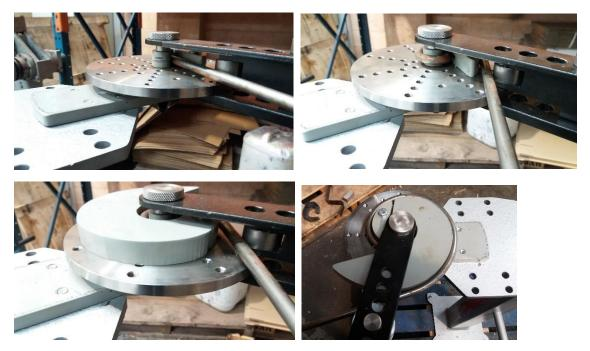
With normal bending of steel, a 12mm Diameter pin is used (minimum radius) or the stepped pin with 3 sizes of rollers to get desired bend radius.
