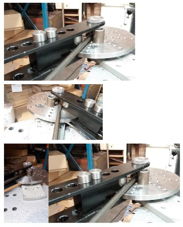
The inspiration behind this design was based on the Blacksmiths Wheel where hot steel was heated and bent around a pin set on a Disc like this.
