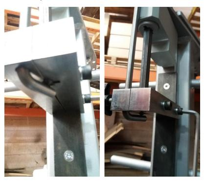
Twist is now performed in desired direction. Twist is now reversed opening out cage to desired shape.
