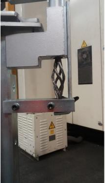
If cage does not open out evenly a large screw driver or similar can be used between the cage legs to gently even them out before removing cage from top and bottom dies.
