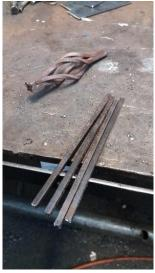
Bar assembly is now inserted into Picket Twister with dies in handle assembly faceing down.
