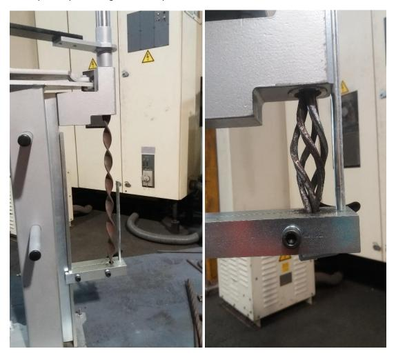
This Picket Twister is Designed to Twist 25mm x 5mm flat mild steel bar or 12mm (1/2inch) square mild steel bar.
